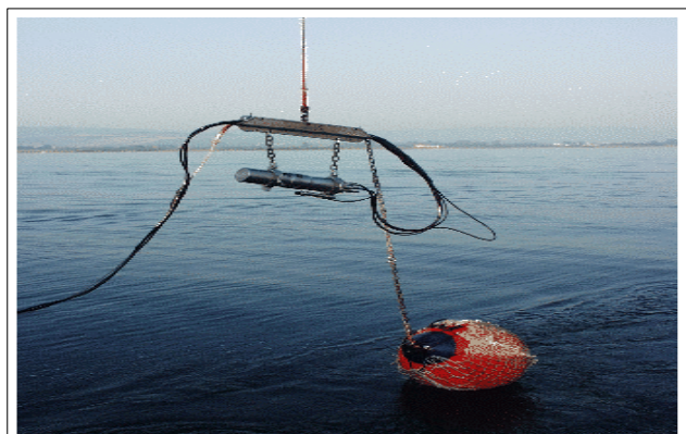
Figure 2-4. Tail buoy (in red) at the end of a 1-2 km streamer being deployed
