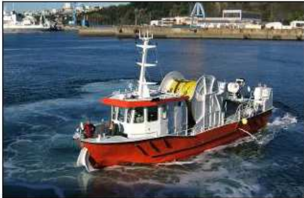
Figure 2-5. Example of a small shallow draft 2-D cable vessel
